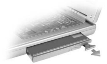
3 Insert the new device into the bay, and push the device until you feel a click.
