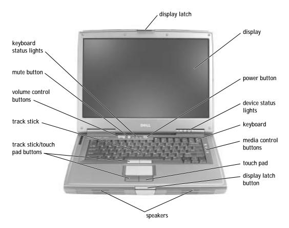
**DISPLAY LATCH** — Keeps the display closed.
