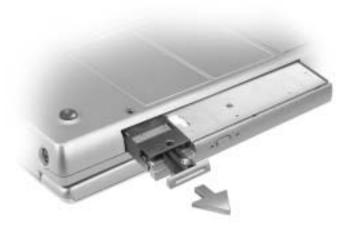
7 Insert the new device into the bay, push the device until you feel a click, and replace the screw.
