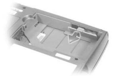
**3** Pull the reserve battery out of its compartment, and disconnect the reserve battery cable from the connector.
