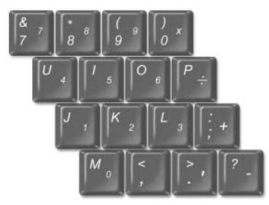
The keypad numbers and symbols are marked in blue on the right of the keypad keys. To type a number or symbol, ensure that the keypad is enabled, and press  $\boxed{Fn}$  and the desired key. The  $\bigcirc$  light indicates that the keypad is active.
