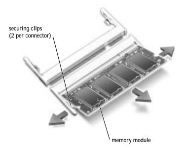
NOTICE: If you need to install memory modules in two connectors, install a memory module in the connector labeled "DIMM A" before you install a module in the connector labeled "DIMM B." Insert memory modules at a 45-degree angle to avoid damaging the connector.
