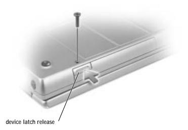
6 Pull the device out of the module bay.
